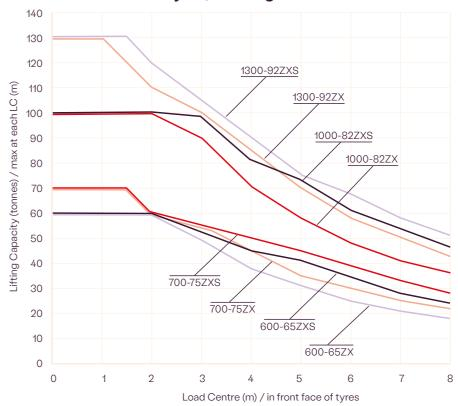
X = capacity without Support Jacks. XS = capacity with Support Jacks (0 km/h).
